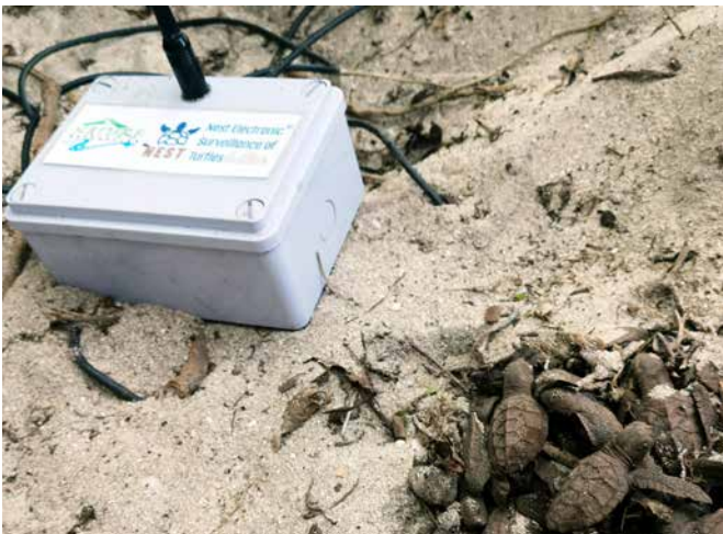
NEST automatically monitors and transmits turtle nest environmental data
